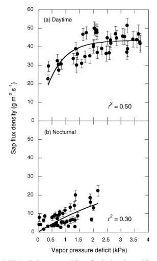
**Fig. 3.** Relationship between mean daily sap flux density and mean daily vapor pressure deficit of mature tamarisk trees (n = 20 trees) in southeastern Utah on days 130–170 during the 2008 growing season. (a) Relationship between mean daytime sap flux density and daytime vapor pressure deficit ( $r^2$  = 0.50, P < 0.0001). (b) Relationship between nighttime sap flux density and nighttime vapor pressure deficit ( $r^2$  = 0.30, P < 0.0001). Error bars are  $\pm$ standard error of the means.
