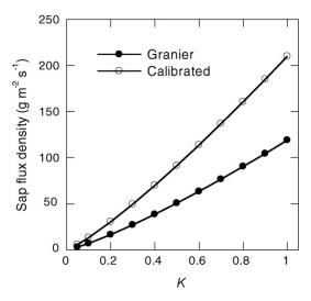
**Fig. 1.** The relationship between sap flux density  $(J_s)$  and K (the ratio between temperature differences during periods of sap flow and temperature differences during zero flow) for Granier calibrated heat-dissipation sensors and lab-calibrated heat-dissipation sensors.
